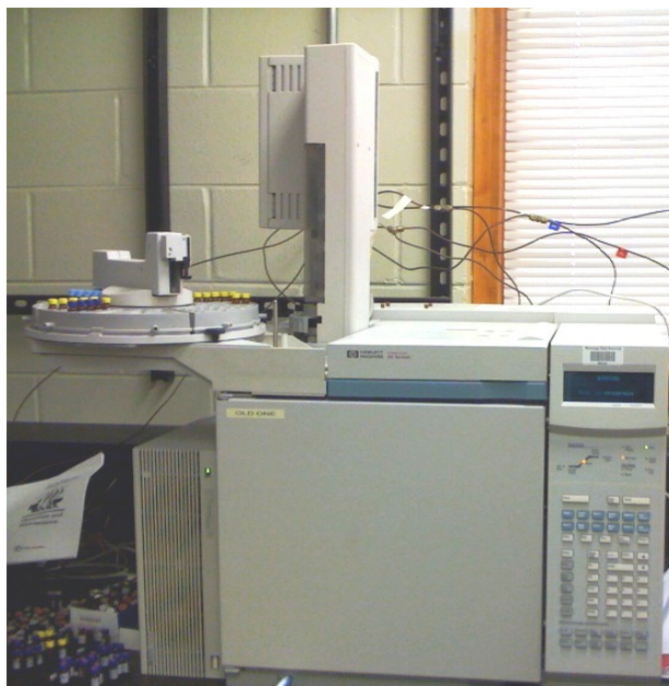
Figure 4.11: The Agilent 6890N gas chromatograph equipped with a flame ionization detector (GC-FID) and autosampler used for FAME analysis (Agilent Technologies, Palo Ato, CA, USA).
