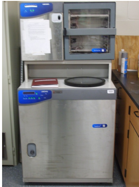
Figure 4.6: Freezone 6 bulk tray freeze-dryer used for the dehydration of cell biomass for cell dry mass determination prior to lipid extraction (Labconco Corp., Kansas City, MO, USA).
