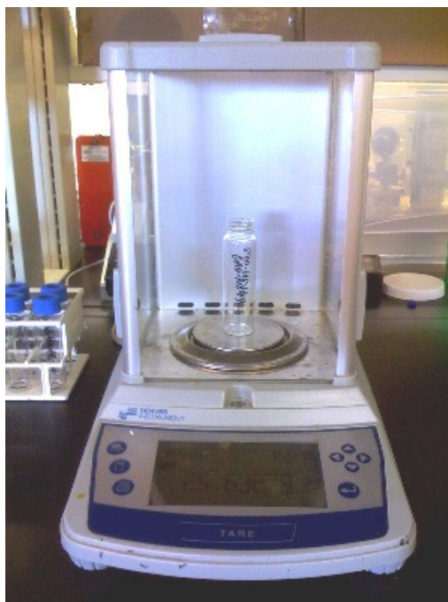
Figure 4.7: Analytical balance used for gravimetric determinations of biomass and lipids in this study (Denver Instrument, Bohemia, NY, USA).
