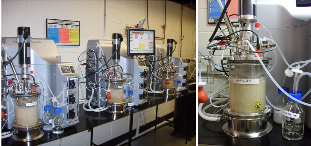
Figure 4.2: BioFlo 310 Fermenters/Bioreactors. LEFT: Set-up showing the master control unit with the VGA touch-screen display in the middle and two utility units on either side. RIGHT: Close-up image of one fermentation unit vessel (New Brunswick Scientific Co., Edison, NJ, USA).
