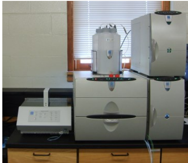
Figure 4.14: ICS-3000 ion chromatograph used for residual ammonium analysis (Dionex Corp., Sunnyvale , CA, USA).
