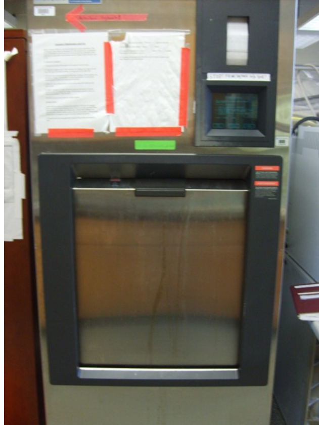
Figure 4.4: Amsco Century SG-120 Laboratory Autoclave/Sterilizer (Steris Corp., Mentor, OH, USA).
