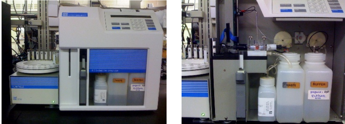
Figure 4.12: YSI 2700 Biochemistry Analyzer used for residual glucose and xylose analysis (YSI Inc. Life Sciences, Yellow Springs, OH, USA). LEFT: Exterior image showing the attached 2710 Turntable. RIGHT: Interior image of the main unit.
